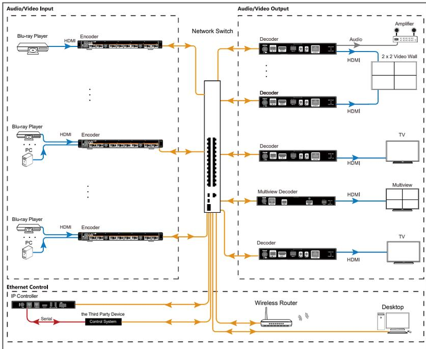
The Multiview processing decoder is used in conjunction with H.264/H.265 encoders and decoders for flexible AV distribution of point-to-point, point-to-multipoint, multipoint-to-point and multipoint-to-multipoint over a Gigabit network.
